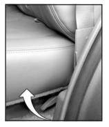
1. Pull up the lever located under the seat cushion. Escalade lever shown, Escalade ESV lever similar.
